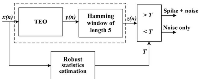
Fig. 1 Block diagram of the spike STEO detection with adaptive threshold.
